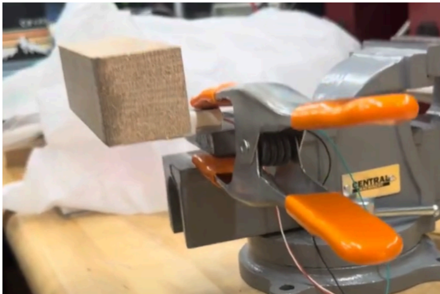
Figure 9.2 - Lab Mass used for load cell prototyping
